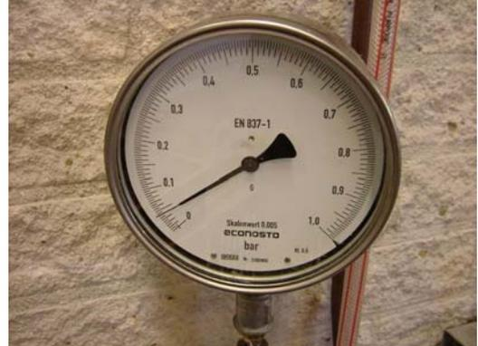
The test pressure is the pressure equivalent to or resulting from filling the test section up to the ground level of the downstream or upstream manhole as appropriate with a maximum pressure of 50 kPa and a minimum pressure of 10 kPa measured at the top of the pipe.
