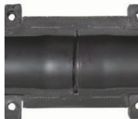
Fig. 8 Section of two pipes joined with Electro Fusion
