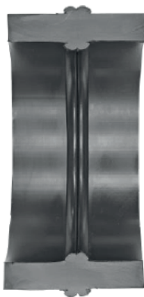
Fig. 3 - Section of a Butt Fusion welded joint
