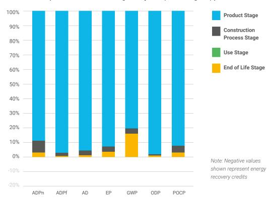
Environmental profile of the PVC-U rain gutter system (cradle-to-grave) per functional unit
