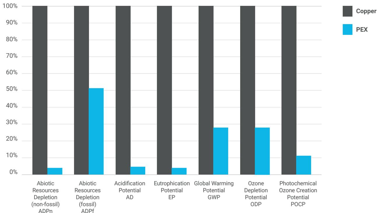
Environmental profile of the PEX pipe system for hot and cold water in the building from cradle-to-grave per functional unit
