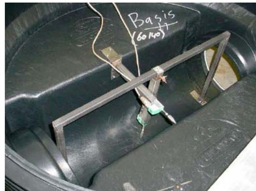
Impression of measuring spots, mid-point deformation and horizontal deformation
