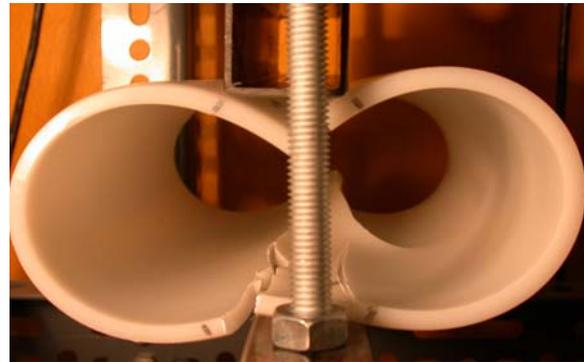
Figure 5. a) Compliance curves for OD10mm PE pipes (aged/un-aged samples), b) Photograph of un-aged PE sample at 45% deflection.
