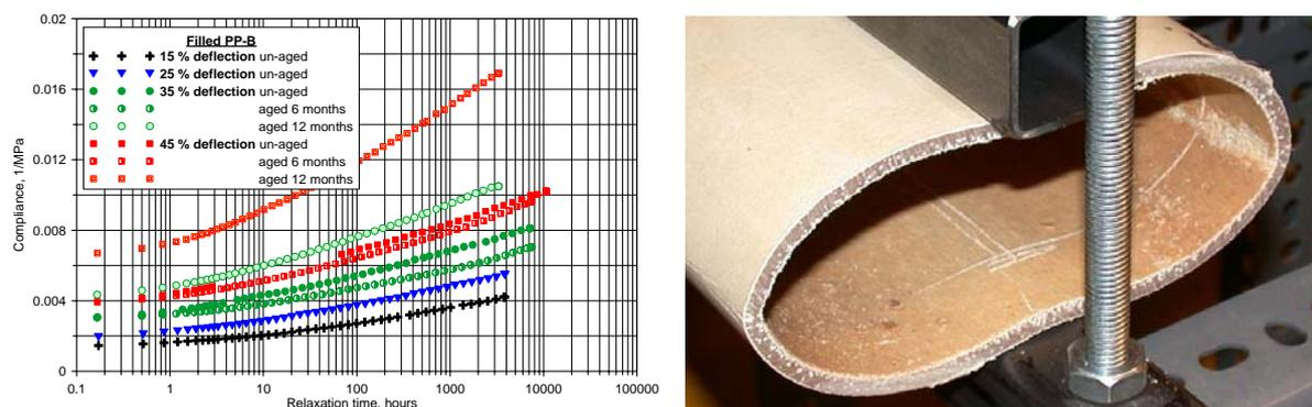
Figure 4. a) Compliance curves for OD110mm filled PP-B pipes (aged and un-aged samples), b) Photograph of sample aged 1 year at 45% deflection.
