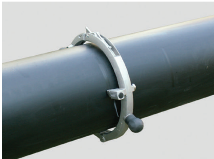
Figure 14: Example of mechanical scraping tool
