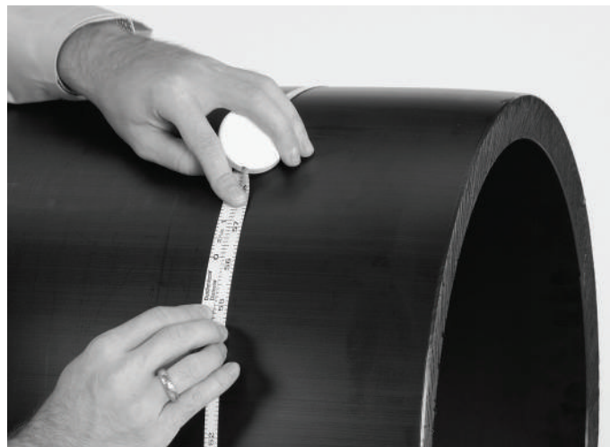
Figure 17: Checking the outer diameter of the pipe
